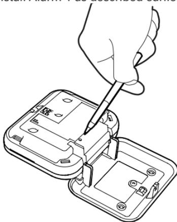
Using a ballpoint pen, briefly push and release the 'learn button' on the back of Alarm 2. The red LED next to the learn button will flash briefly then light up for approximately five seconds.
