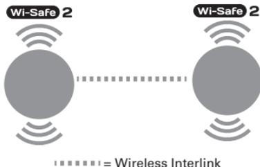
Wi-Safe 2 enables wireless communication with any other product with Wi-Safe 2 technology inside. A wireless transceiver inside every alarm communicates with others by continuously sending and receiving wireless signals otherwise known as a 'meshed network'. When one alarm detects CO the wireless module inside sends a radio frequency signal to all the connected alarms, ensuring almost instantaneous reaction across the entire network.
