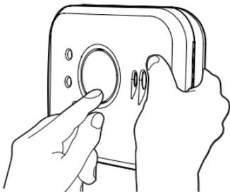
The red LED on Alarm 2 will flash to indicate that it has been 'learned-in' successfully. If the test button is not pressed quickly enough, the 'learn-in' process will fail. If this happens, repeat the process. To complete the installation fit Alarm 2 into position.
